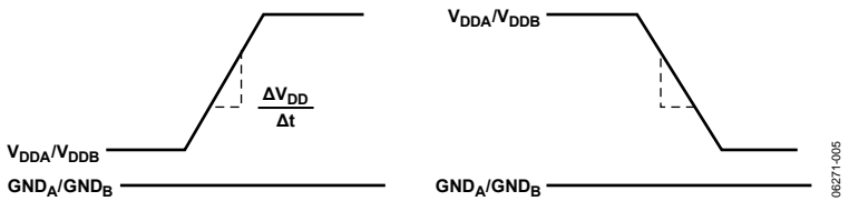
Figure 13. Transient Immunity Waveforms—Output Supplies
